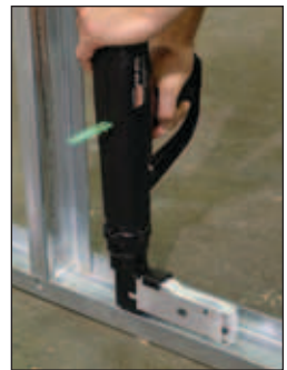
Rotating magazine allows for installation flexibility
