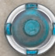
WHEN PROPERLY SET, ANCHOR INDICATOR WILL LEAVE BLUE PAINT IN RECESSED CAVITIES
